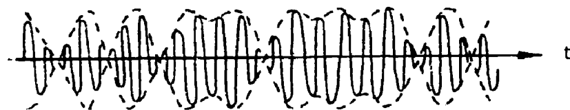
Fig. 3. Binary DSB or PRK signal
